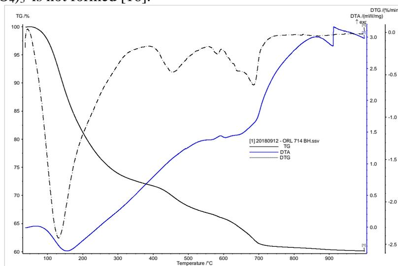
**Fig. 1.** TG, DTG, DTA curves for Rosia Montana, Orlea 714 mineral sample
