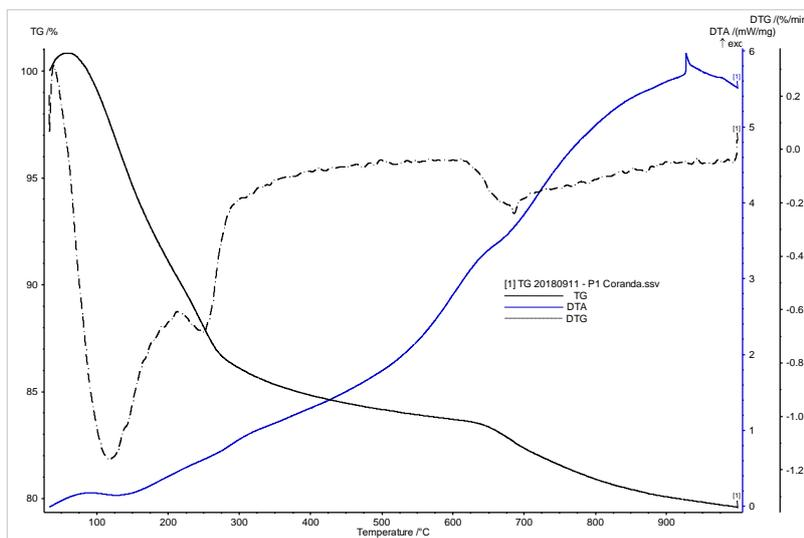
**Fig. 2.** TG, DTG, DTA curves for Certej P1Coranda mineral sample
