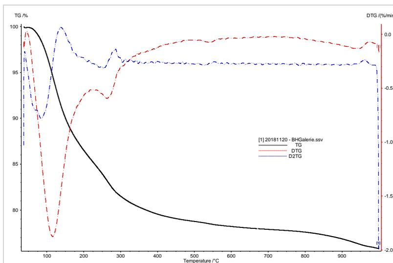
**Fig. 3.** TG, DTG, D2TG curves for Boita Hateg Orizont 120 mineral sample
